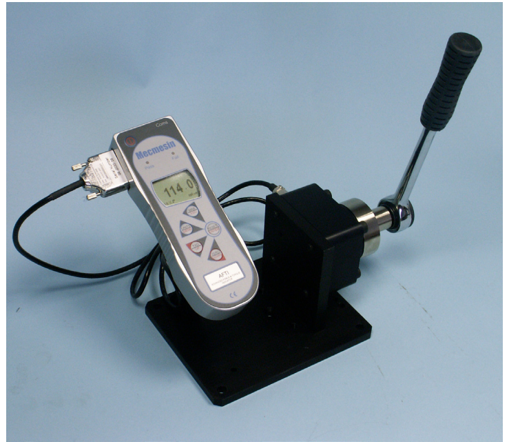
TWC shown testing a mechanical torque wrench
